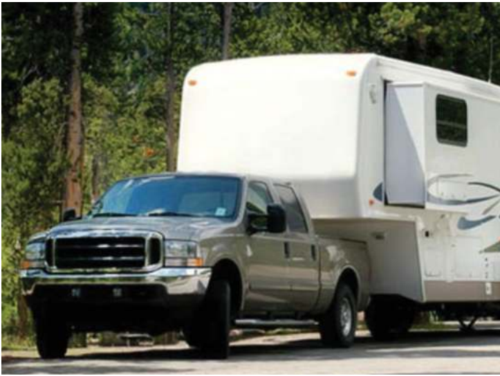
Fifth Wheel Trailers have a modified hitch that attaches to the flatbed of a pickup truck
